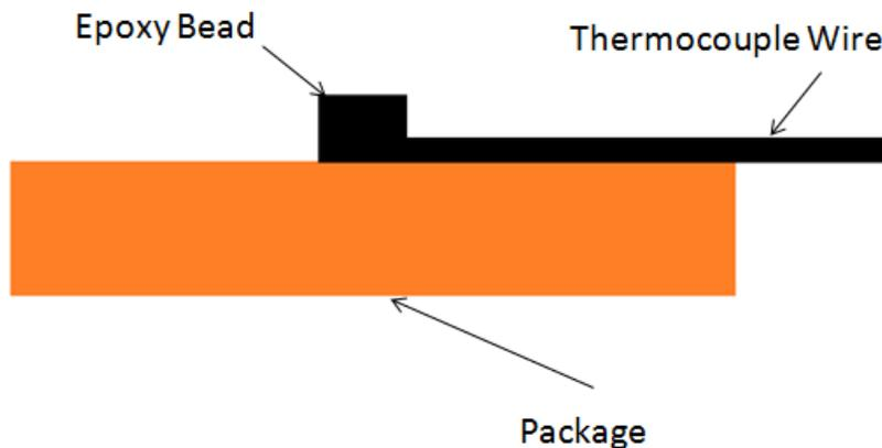
**Figure 13-26. Technique for Measuring  $T_{\text{case}}$  with  $0^\circ$  Angle Attachment, No Heat Sink**
