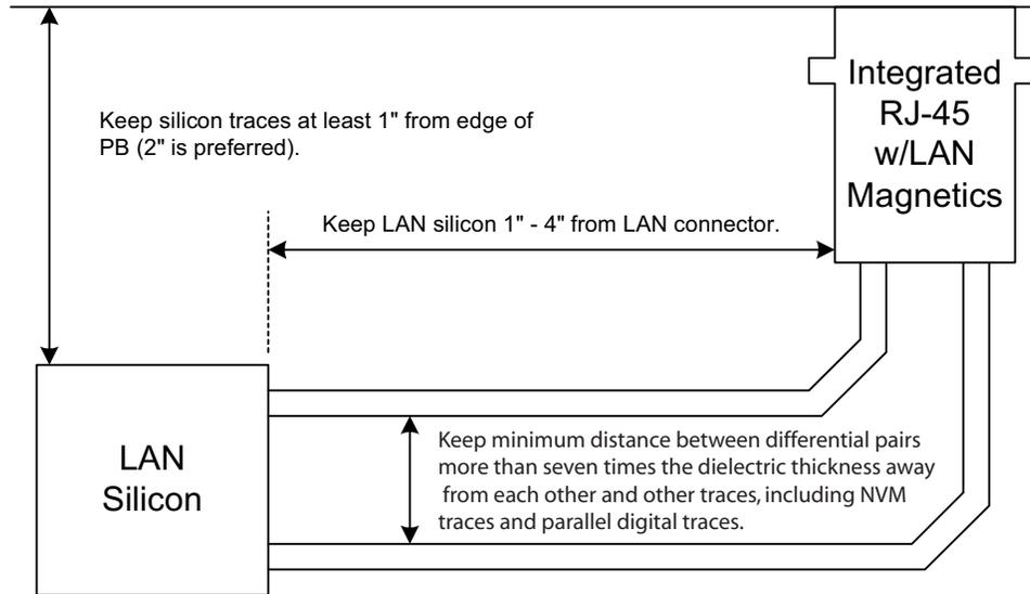
**Note:** Figure 12-13 represents a 10/100 diagram. Use the same design considerations for the two differential pairs not shown for gigabit implementations.
