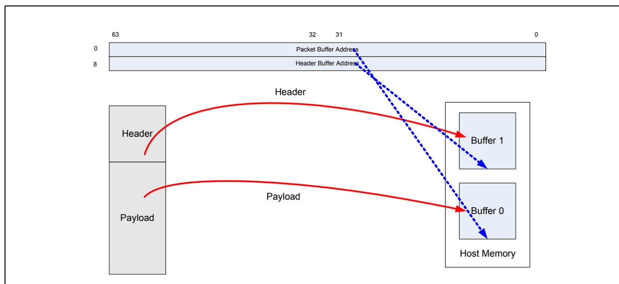
**Figure 7-8. Header Splitting**
