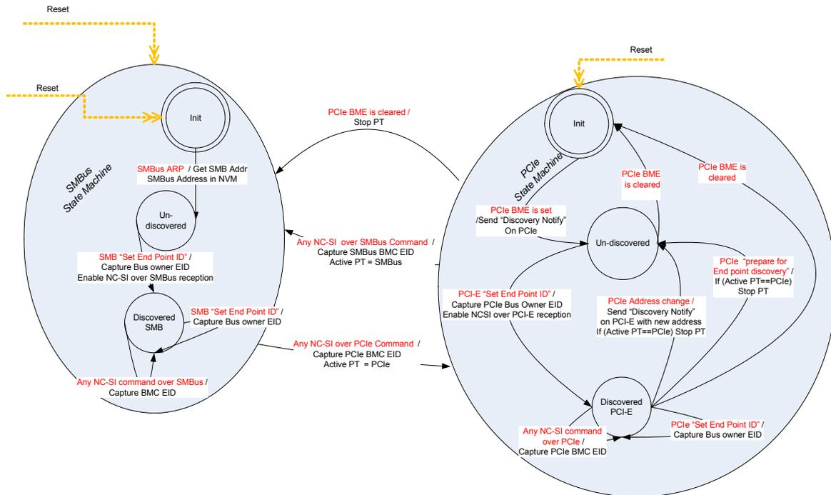
**Figure 10-10. MCTP Bus Transition State Machine**
