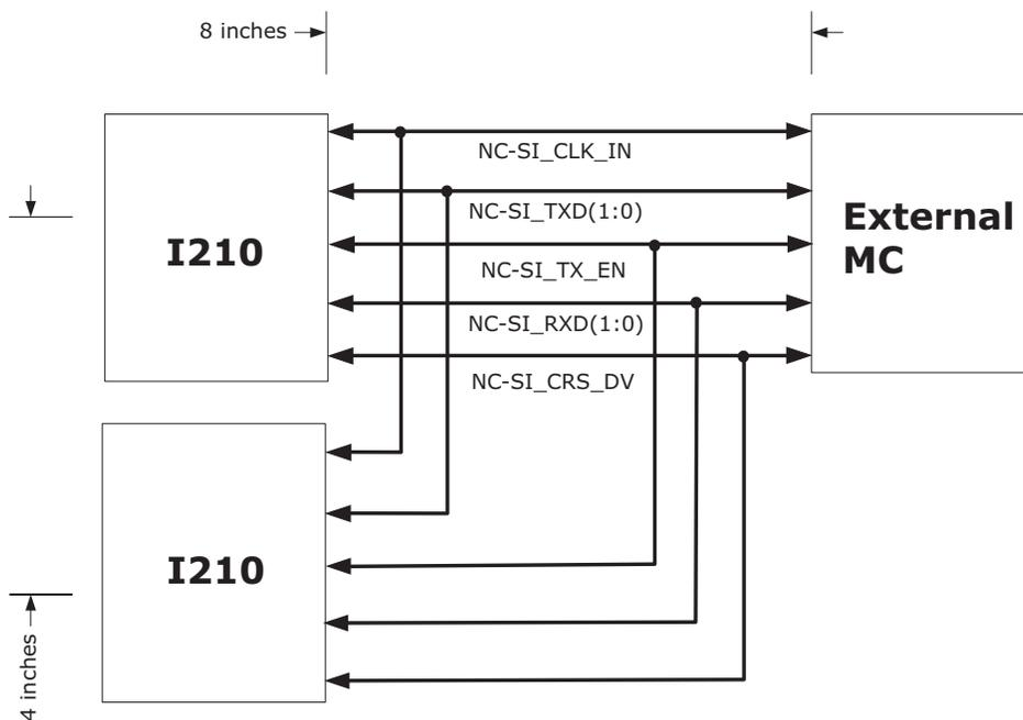
**Figure 12-20. NC-SI Trace Length Requirement for Multi-Drop**
