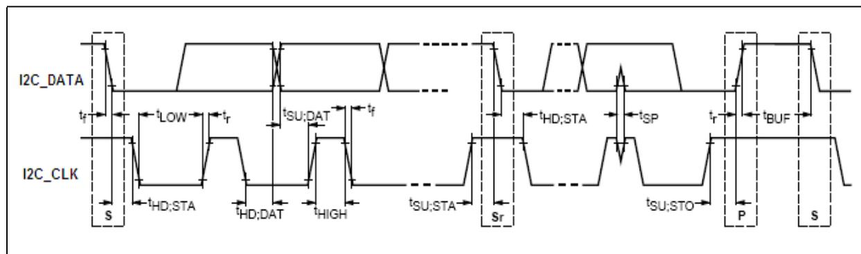
**Figure 11-3. I<sup>2</sup>C I/F Timing Diagram**
