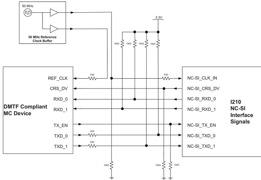
Figure 12-16. NC-SI Connection Requirements - Single-Drop Configuration
