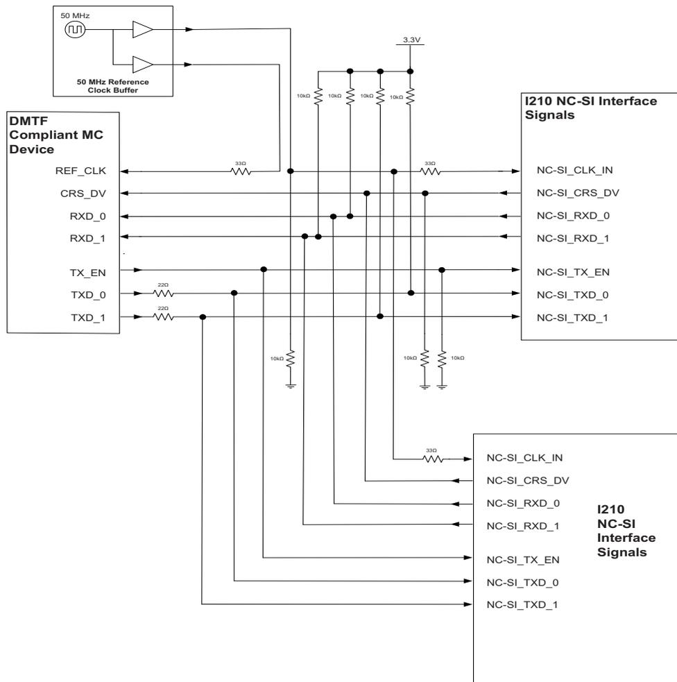
Figure 12-17. NC-SI Connection Requirements - Multi-Drop Configuration
