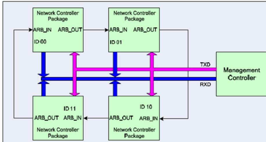
**Figure 12-18. NC-SI Connection Requirements - Hardware Arbitration**
