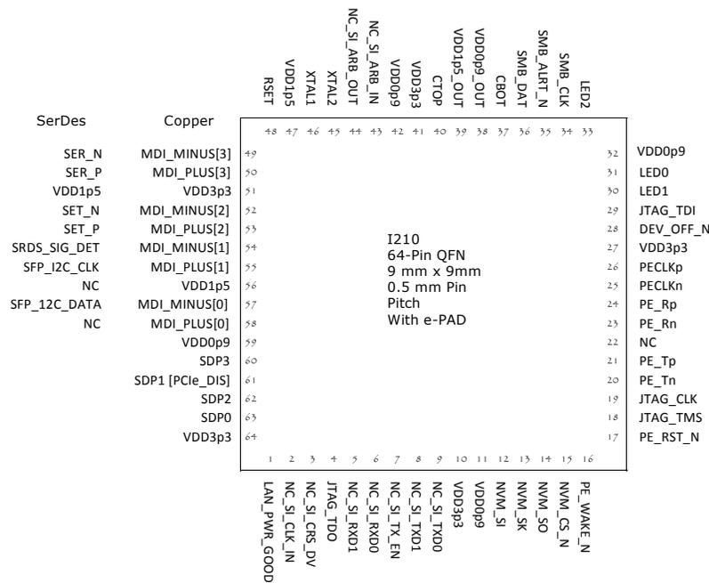
Figure 2-1. I210 64-Pin, 9 x 9 QFN Package With e-Pad
