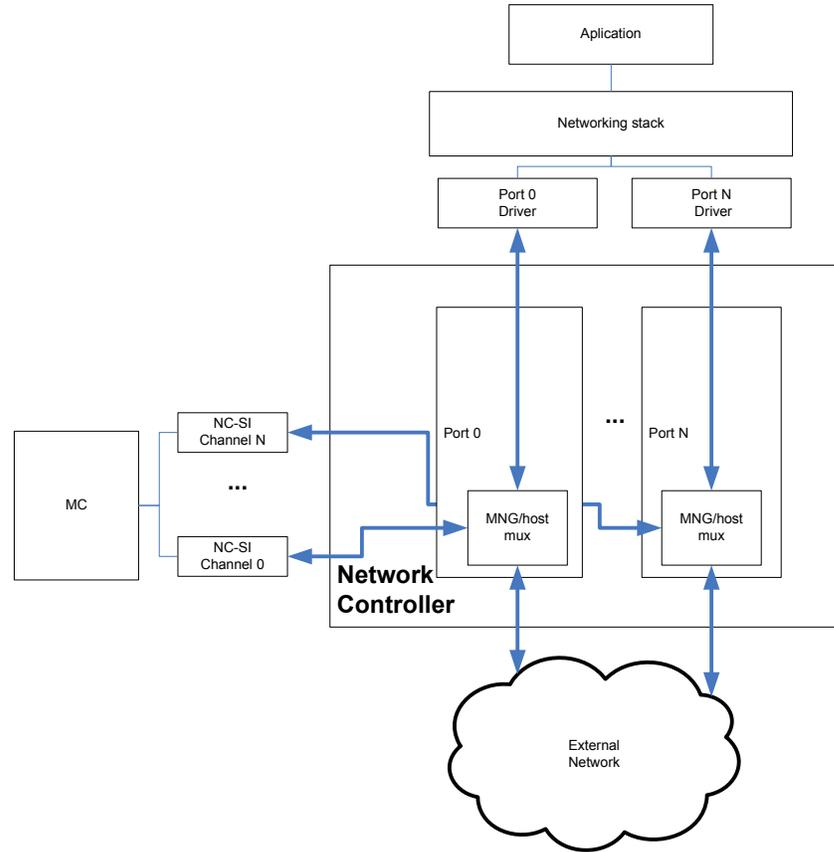
**Figure 10-2. OS-to-MC Diagram**
