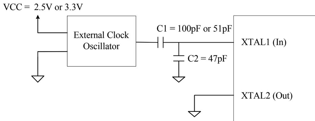
**Figure 11-9. External Clock Oscillator Connectivity to The I210**
