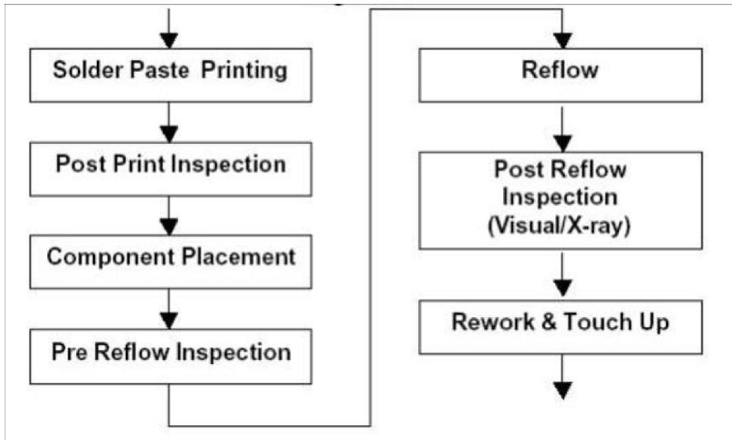
Figure 12-25. Assembly Flow
